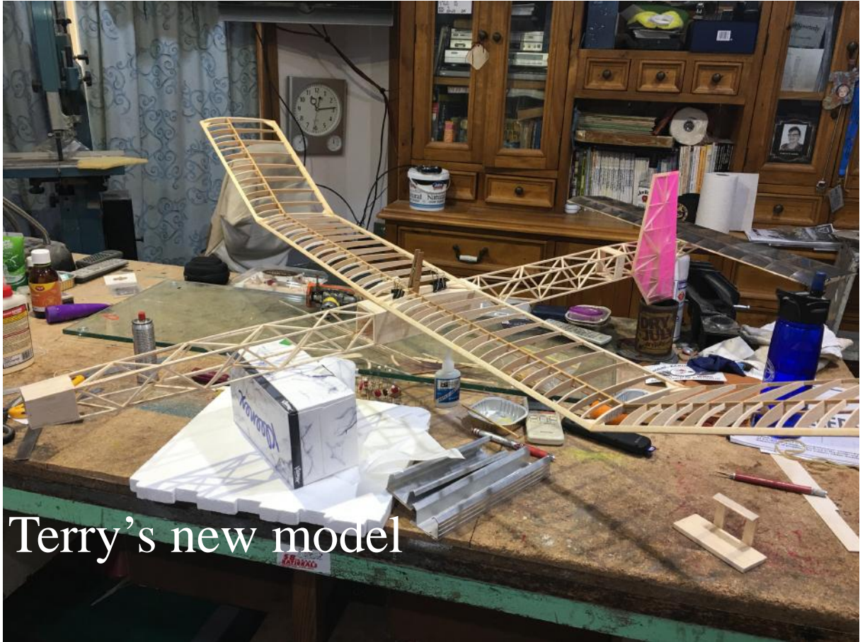
Slowly getting there. Covering, prop and front end to go. A proper open rubber model.
